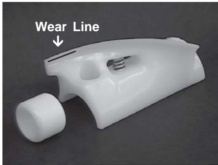
Figure 16. Auger Flight Wear & Front Auger Support Bushing Wear
